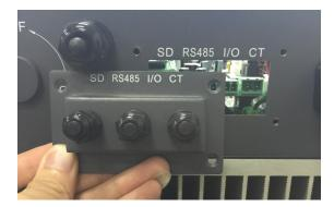
Step 3: Insert the other end of Network cable through the cable gland and waterproof.
