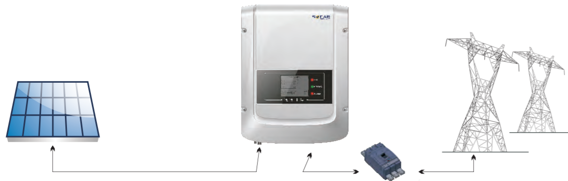
Figure2-1 PV Grid-tied System
