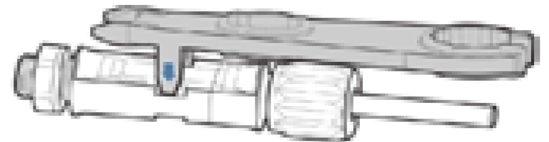
Figure 4-18 Removing a DC input connector
